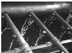
**5.** R130 adapters are thermally welded to branch arms. Bayonet style nozzles snap into place with just a quarter turn.
